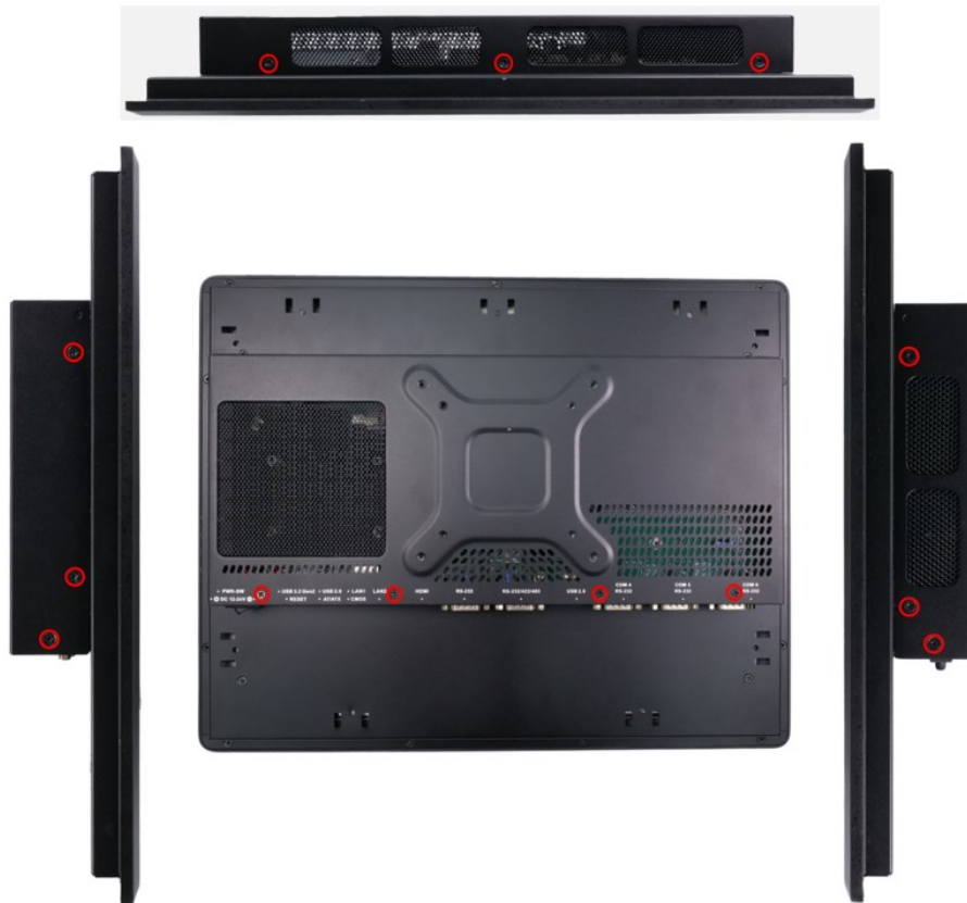
Figure 3-1: PPC2-Cxxx-EHL Back Cover Retention Screws
