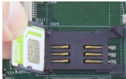
Insert Mini-SIM card with pins facing up
