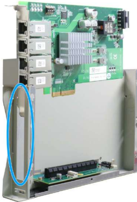
Remove bezel cover and insert the card
