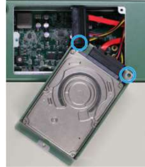
HDD/SSD tray installation orientation
