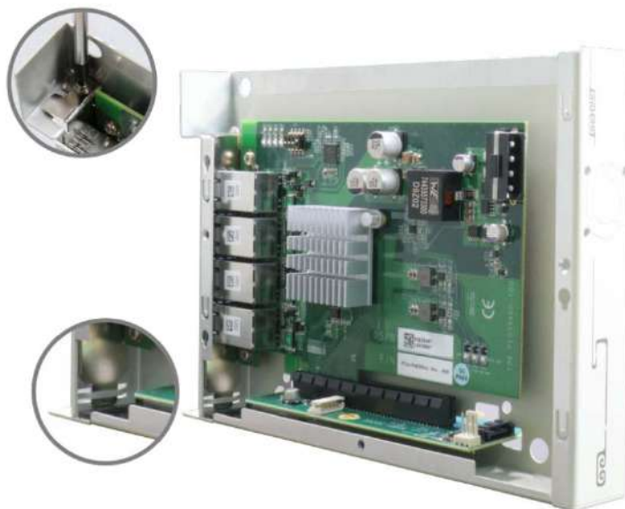
Remove bezel cover and insert the card
