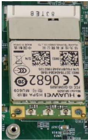
Insert on 45 degree angle
