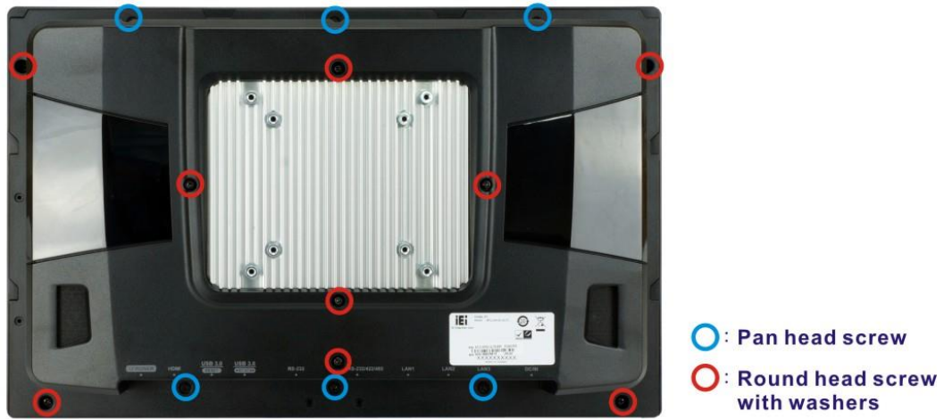
Figure 3-1: AFL3-W15C-ULT5 Back Cover Retention Screws
